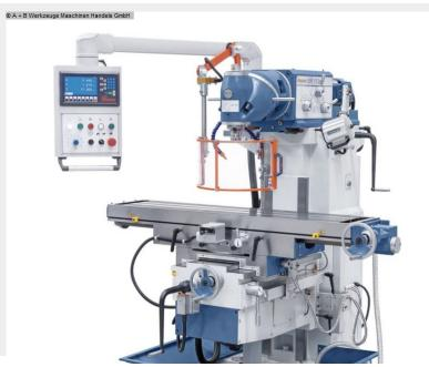
The universal milling machine UWF 110 Servo is suitable for the execution of light and medium-heavy milling work. Thanks to their great versatility and It can be used in workshops for machining small and simple conversions medium-sized series can be used successfully. Special features of this The machine is the swiveling work table, the flat guide in the y and z axes and the servo drive for feeds and rapids in all axes.
